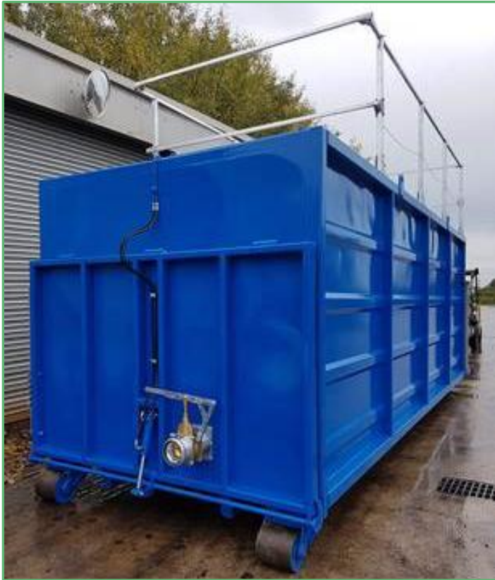
Left: Rear view of the STU showing the hydraulic actuating rear door and sludge extraction point.
