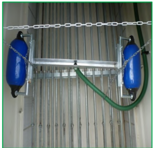
Left: The internal view showing the unique heater coils, access ladder and floating oil skimmer, along the base can be seen the water removal filter screen system.
